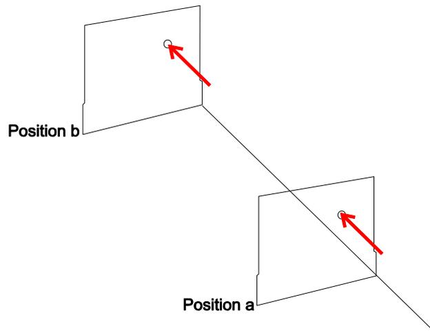
The CoSy head has to be positioned such that the laser beam falls into the input aperture exactly vertically. The laser beam must be polarized vertical to the tabletop plane.
