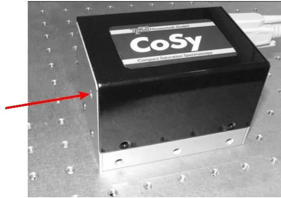
Fig.. 1.2 The CoSy measurement head
