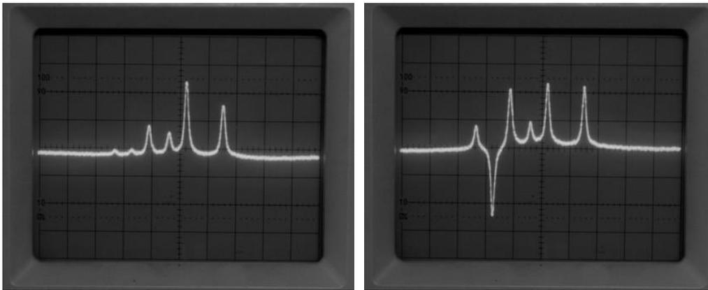
Fig. 7.1: The same doppler-free saturation spectrum of Rb with and without a magnetic field at the location of the glass cell.
