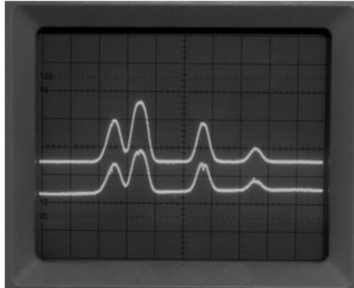
Fig. 6.2 Oscilloscope screen with laser on (here: rubidium D2 lines)
