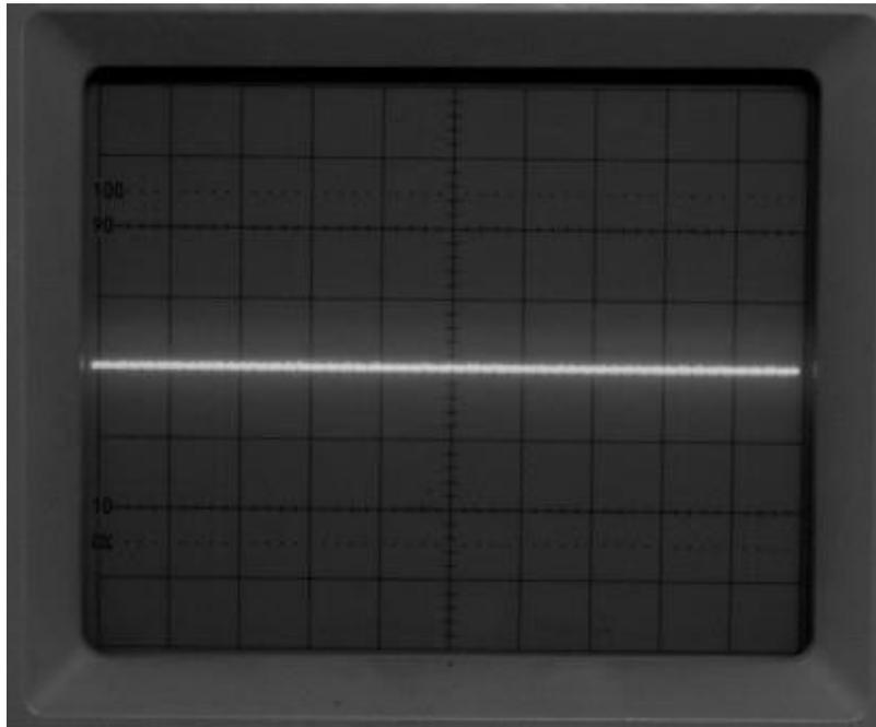
Fig. 6.1 Oscilloscope screen after dark current adjustment
