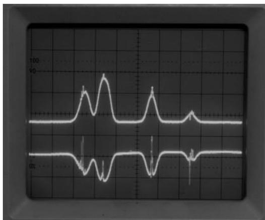
Fig. 6.4: Absorption signals with clearly visible hyperfine structure
