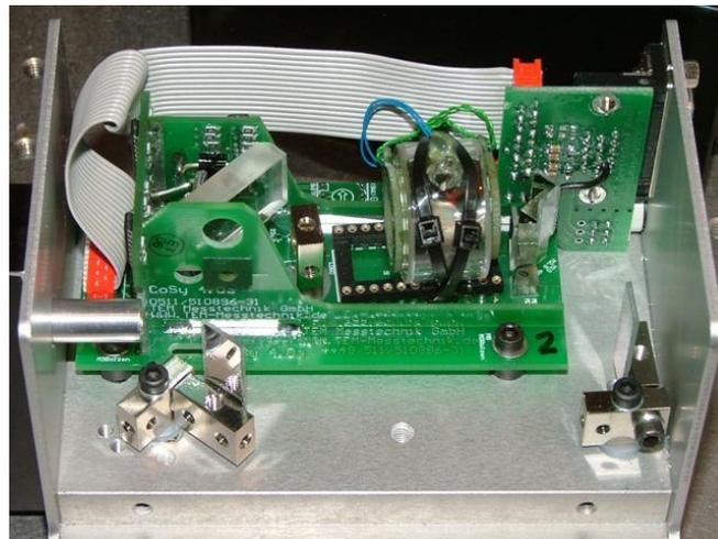
Fig. 1.3 The CoSy measurement head from the inside
