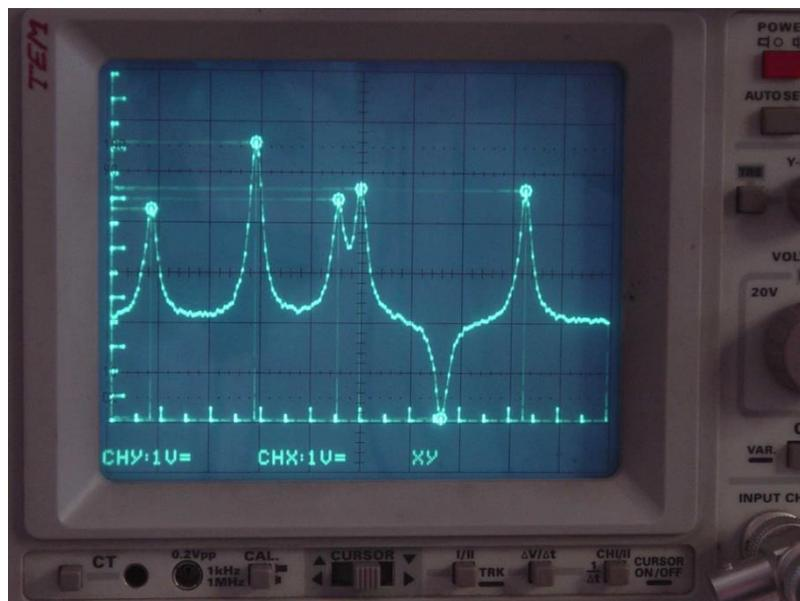
Fig. 1.1 Doppler-free saturation spectrum of the Cs-D<sub>2</sub>-absorption line
