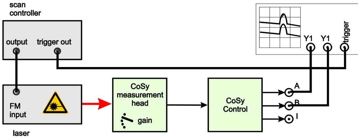
Fig. 4.1: diagram of connections
