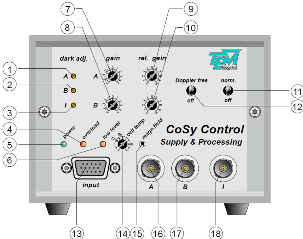
Fig. 3.2.2.1 Control elements on CoSyControl front panel
