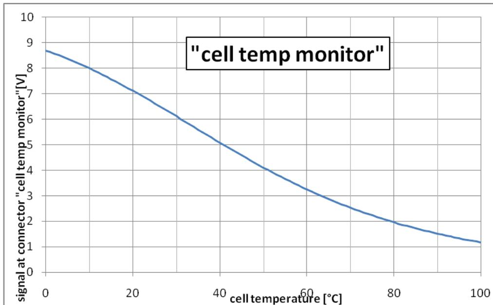
Fig. 8.2.1: signal at connector cell temp monitor vs. cell temperature
