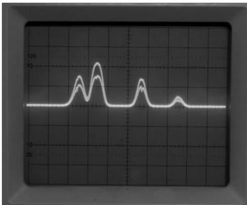
Fig. 6.3: Signals A and B without offset after gain adjustment
