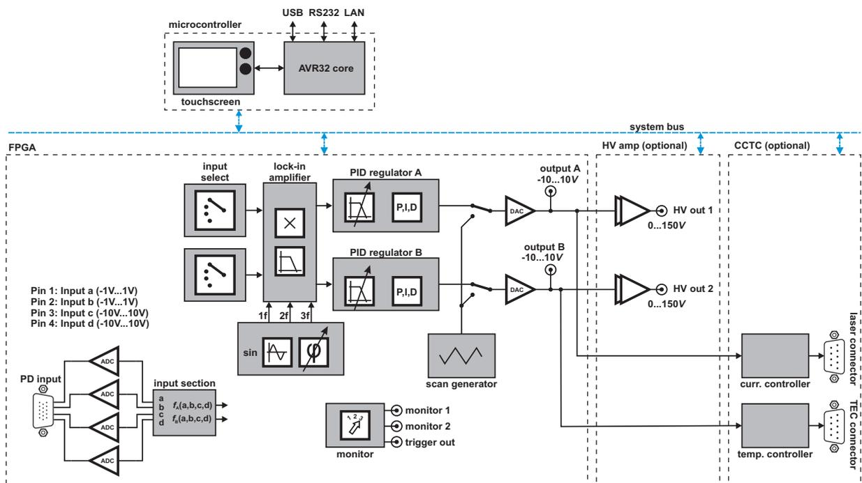
Figure 3: Schematic block diagram of *LaseLock* device
