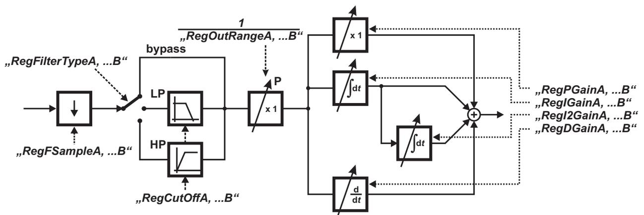
Figure 28: PID regulator with filter
