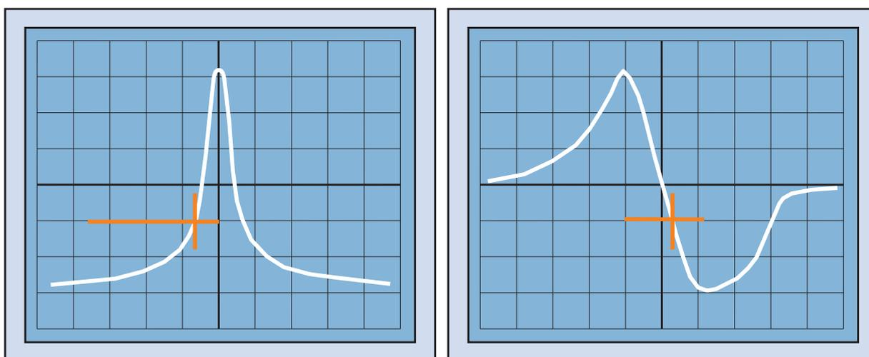
Figure 1: Side-of-fringe stabilization
