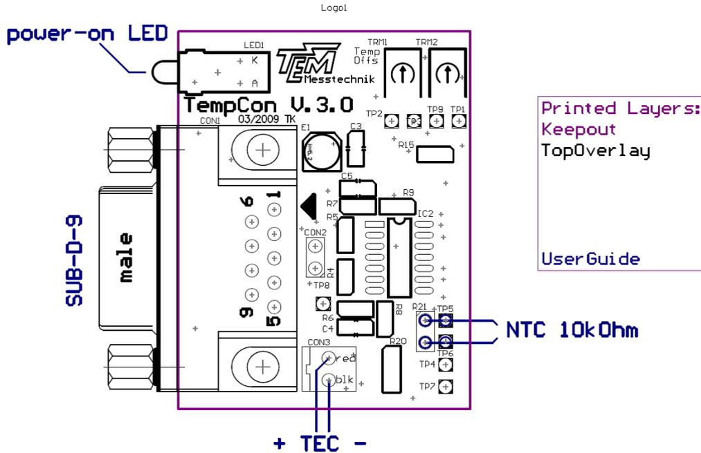
Figure 15: Temperature sensor amplifier board
