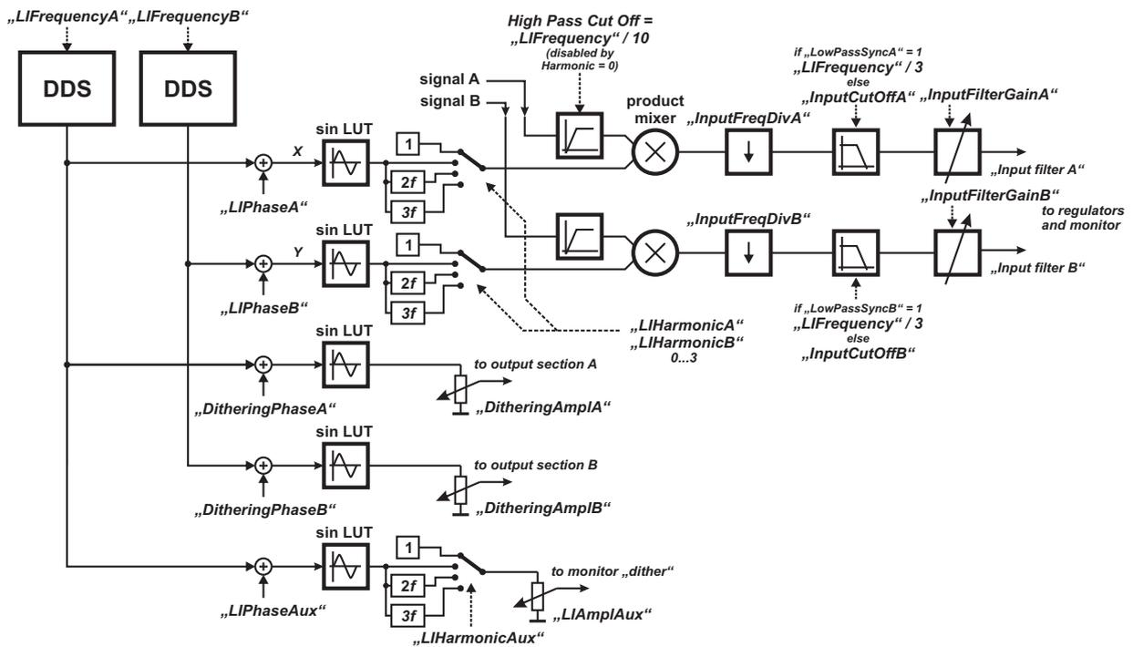
**Figure 23:** Block diagram of the lock-in amplifier section
