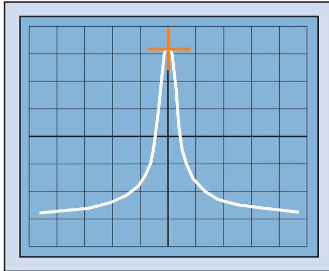
**Figure 2:** Top-of-fringe stabilization
