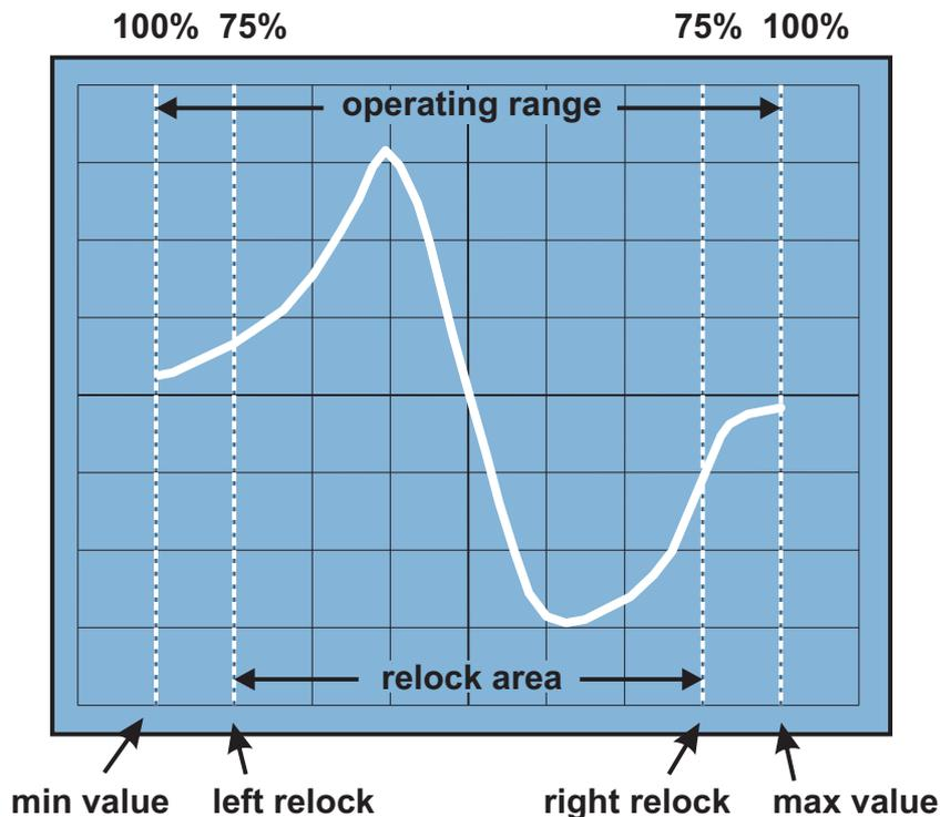
**Figure 26:** Display of the input signal vs. the output signal, which is applied to the controlled system. Explanation of the operating range and the relock range (example: relock = 75%)
