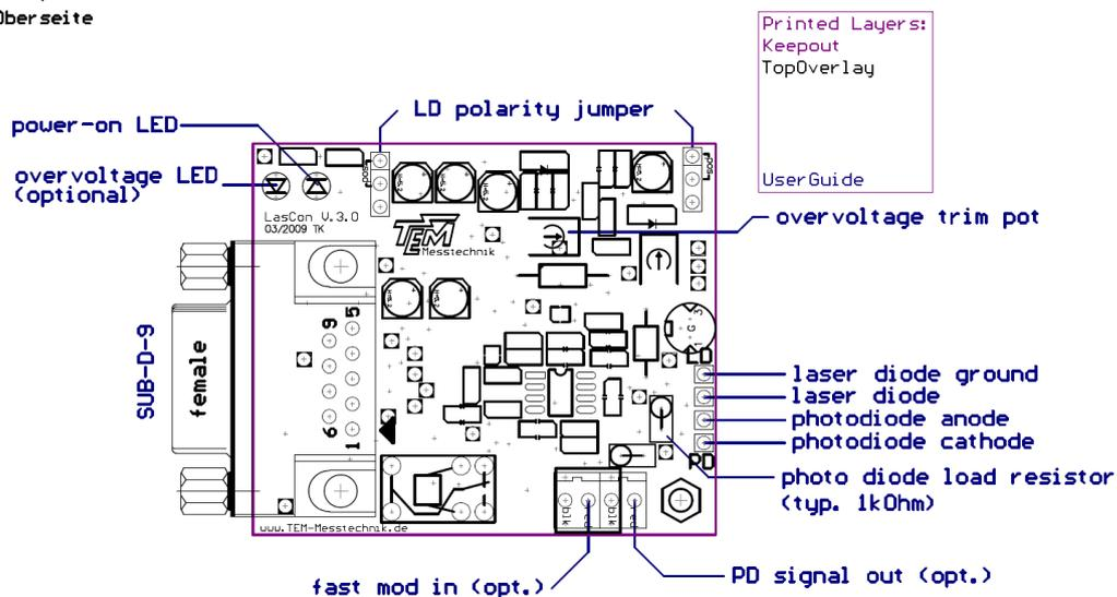
Figure 16: Laser modulation board
