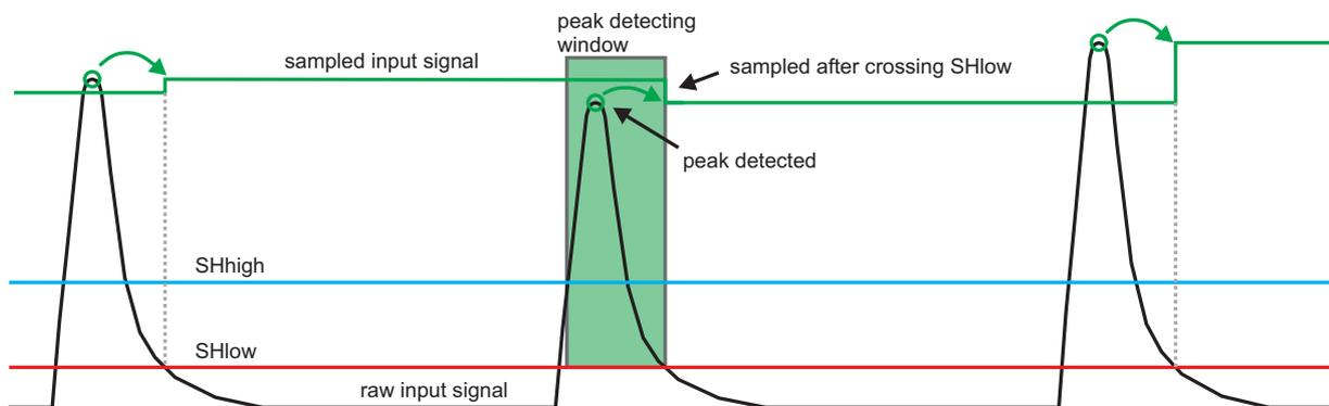
**Figure 22:** Principle of sample and hold stage
