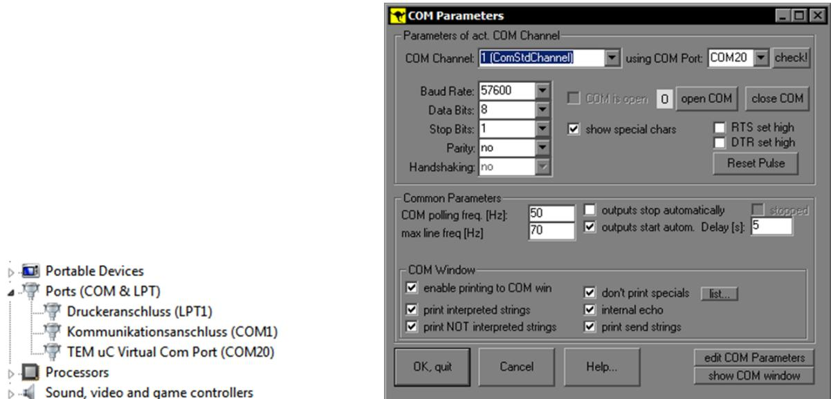
**Figure 17:** COM Port in the device manager (left) and corresponding COM port settings in Kangoo (right)
