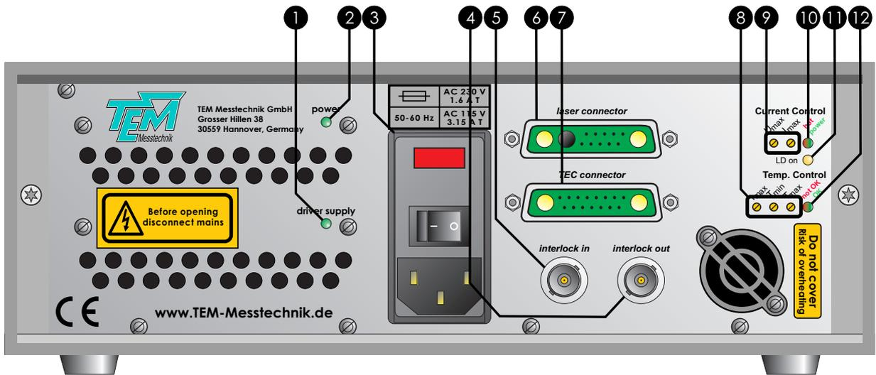
Figure 9: Rear panel elements (CCTC-12A version)
