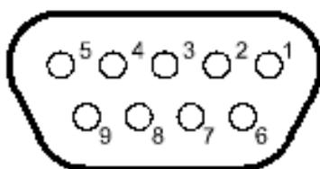
**Figure 14:** Sub-D-9 "laser connector" pinout
