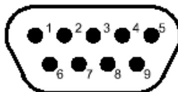
Figure 13: Sub-D-9 "TEC connector" pinout
