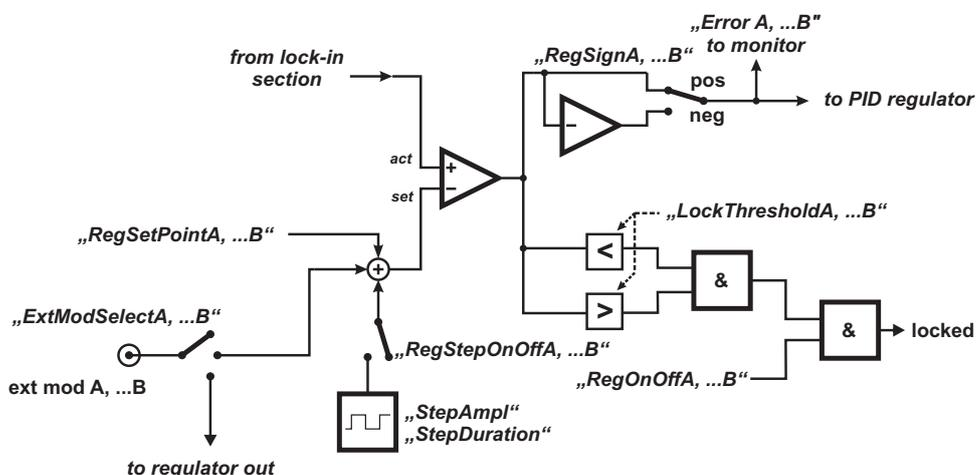
**Figure 24:** Block diagram of the set point section
