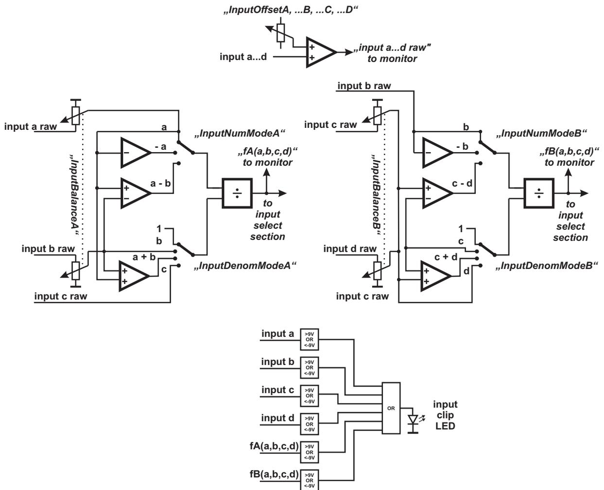
Figure 21: Block diagram of the input section (simple mode)
