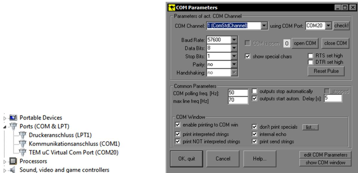
**Figure 32:** COM Port in the device manager (left) and corresponding COM port settings in Kangoo (right)
