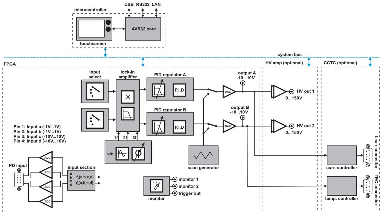
Figure 20: Schematic block diagram of *LaseLock* device
