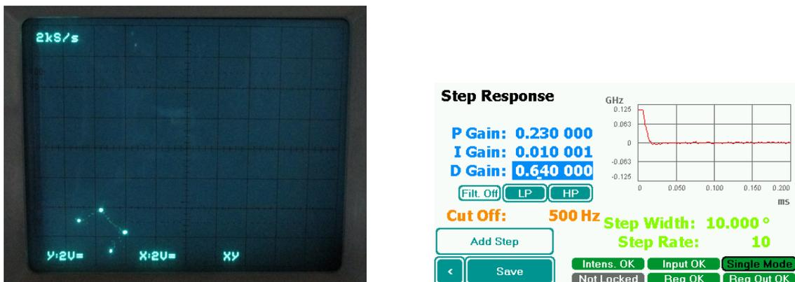
**Figure 27:** A square signal is added to the setpoint resulting in fast steps (outer trace on the oscilloscope, left hand side). The actual value cannot yet follow the steps because the integrator is too slow (inner trace on left hand side, red trace on the TFT).
