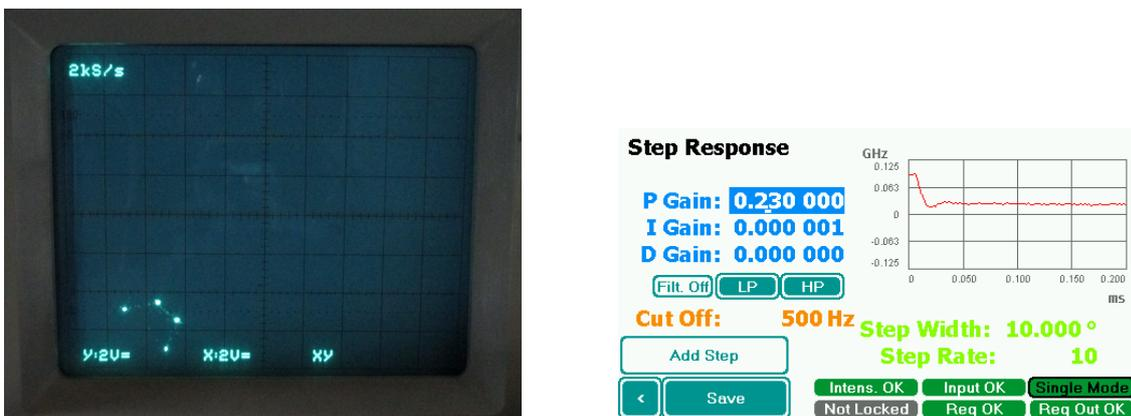
**Figure 25:** A square signal is added to the setpoint resulting in fast steps (outer trace on the oscilloscope, left hand side). The actual value cannot yet follow the steps because the integrator is too slow (inner trace on left hand side, red trace on the TFT).
